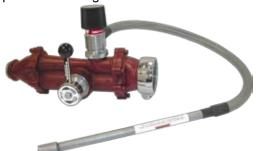
Use a sledge hammer to drive the piercing applicator through concrete block, etc.. Designed to get water or foam to hidden trouble spots. Driving button and point made of hardened tool steel. Impinging jets for a more dense fog pattern. Compatible with Class A and B foams. 1-1/2" F NST swivel inlet. Specify 3' or 6' lengths when ordering. Flow rate of 125 GPM.
