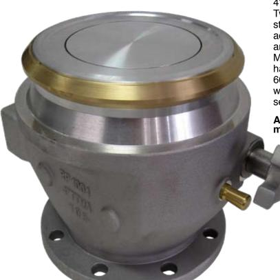
4" Adapter Openable - Bottom Loading Two pieces heat-treated aluminum construction with a hard coated rotatable adapter. One-piece heavy-duty poppet and stainless steel trim for longer life. Multi-position short stroke aluminum handle with smooth rotation of less than 60°. Meets API RP-1004 specifications with a standard 4" TTMA flange. Viton\* seals.
