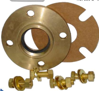
336-L Shore connection is for use with 336-S Ship Connection. The International Shore Connection is a standard 2-1/2" 150 lb. ASA flange drilling. The flange has a 2-1/2" female fire hose thread (NST/NH) to match fire hose threads on the ship. The flange has 4 holes with Bolt Circle Diameter of 5-1/2", the Outside Diameter is 7". The International Shore Connection is supplied with bolts, nuts, washers, and gasket.
