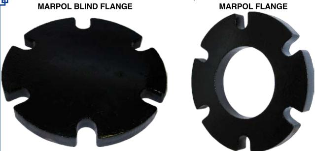
**Marpol Flanges:** are available in pipe ID sizes ranging from 2" to 5" ID, have 6 slotted holes, 7" flange PCD, and 8-1/2" flange OD. Marpol flanges are typically used for oil discharge and/or sewage discharge. The flange is constructed of carbon steel.
