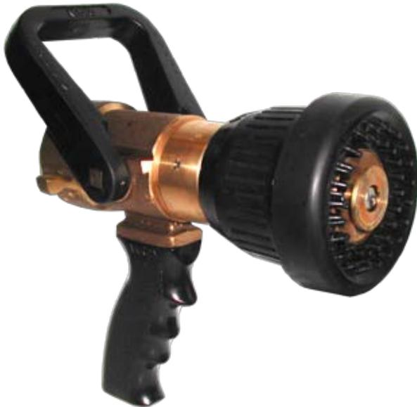
**No. AKRON-3020 - Coast Guard Nozzle**, 1-1/2" F NST inlet; Approval No. 162.027/15/0. A combination fog and straight stream nozzle designed for more efficiency with AFFF or water on-board ships. Brass construction, molded teeth, rubber like bumper and handle, constant gallonage in all FOG and straight stream patterns, flush without shutting down, 95 GPM.
